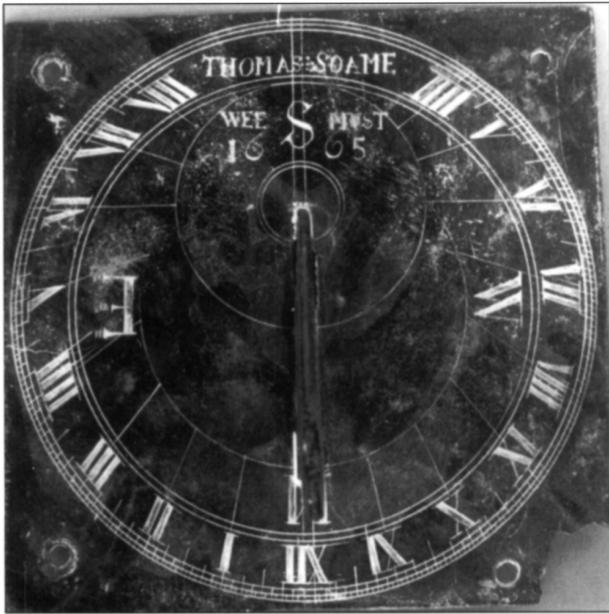
Fig. 1. General view of the dialplate. Note that the dial has been sprinkled with talcum powder to enhance the engravings - in real life, the whole dial is very dark.
