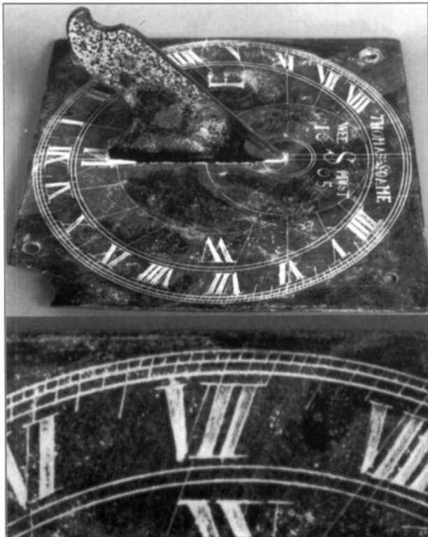
Fig. 2. (Top) View of the dial showing the curious hooked gnomon. (Bottom) A view of the chapter ring showing the neat sixteenth-hour divisions.
